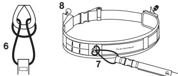
Attach red leash cord with a girth hitch (6) through small red loop on belt (7). Pull yellow ball to release belt and leash (8).
